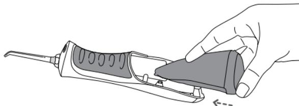
To replace the reservoir on the power handle, simply slide it up towards the top of the unit. The reservoir will snap into place when fully engaged.
