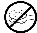
Pipe tape is not recommended.
