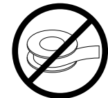
Pipe tape is not recommended.
